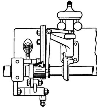
FIG. XI.—6. Variable quality governing by "Conical Cam."
