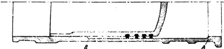
FIG. XII.—32. Wear of Liner due to Piston Movement.
