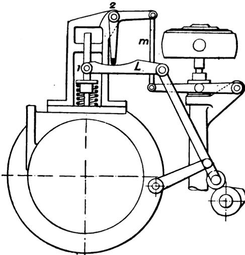
FIG. XI.—14. Gasmotoren Fabrik Deutz variable Valve Lift Device.
