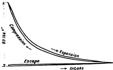
FIG. XIV.—16. Compression Diagram from Engine with cold walls.
