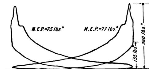
FIG. X.—49. Indicator diagram from double-acting Deutz Engine.
