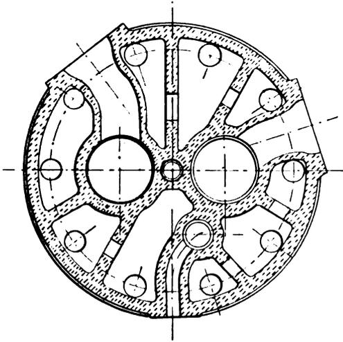
FIG. VI.—4. Section of Cylinder Cover (Diesel Engine).
