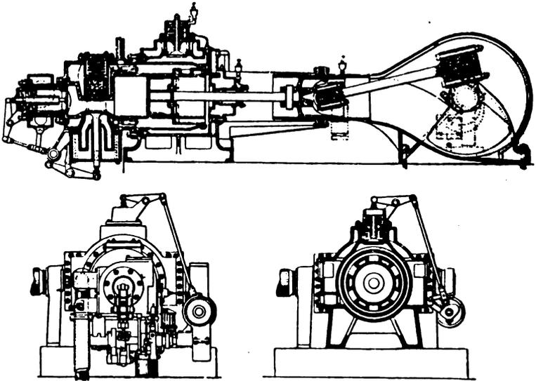
FIG. IX.—1. Clerk supercompression Engine.
