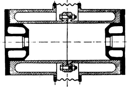
FIG. XII.—54. Section of Cylinder, Snow Steam Pump Works.
