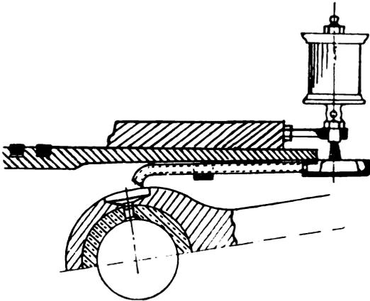
FIG. X.—40. Piston-pin Lubricator.
