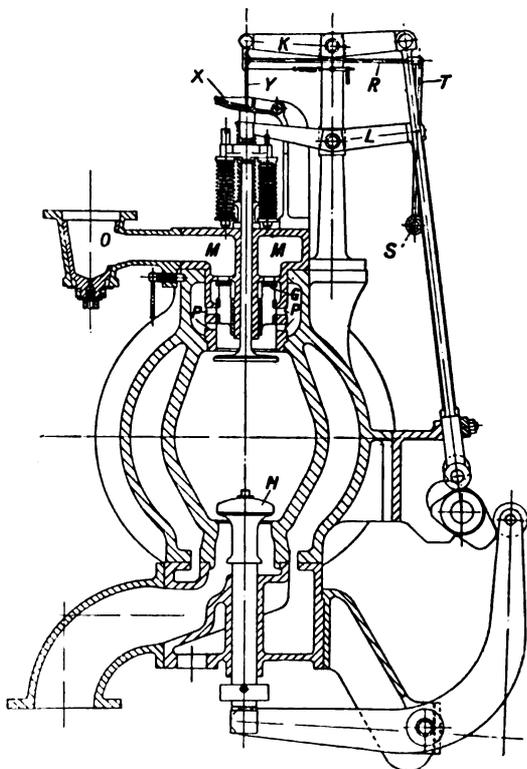
FIG. XIII.—76. Valve Gear of Premier Engine.
