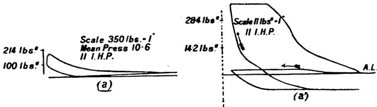
FIG. XV. -31. “Power” and “Resistance” Diagrams, light load.
