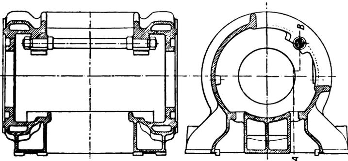
FIG. XII.—58. Intermediate casting or distance piece, Koerting.
