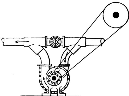
FIG. X.—33. Water circulation by Centrifugal Pump.
