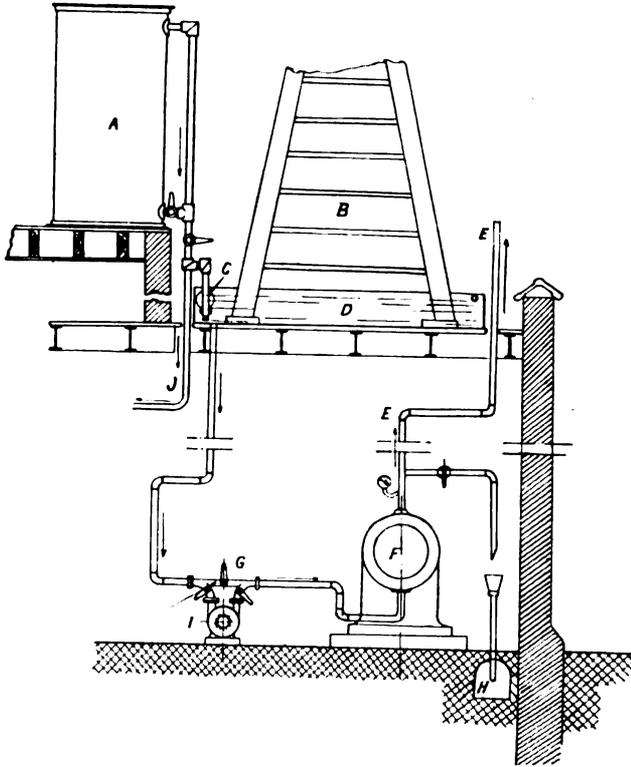
FIG. X. 35. Water circulation (closed system) with cooling apparatus.
