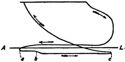
FIG. XV.—8. Re-aspiration of Burnt Products during Suction Stroke.
