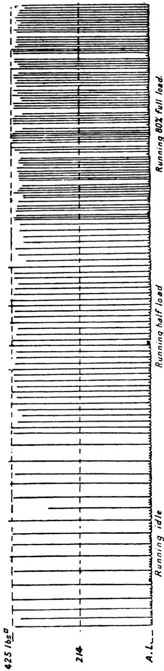
Fig. XV.—27. Explosion Record from "Banki" Benzene Engine.
