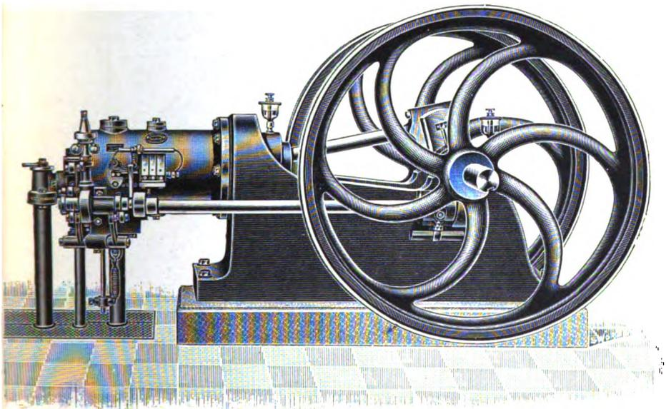
FIG. V.—2. Gas Engine typical of British construction.
