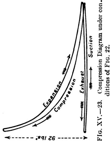
Fig. XV.—23. Compression Diagram under conditions of Fig. 22.
