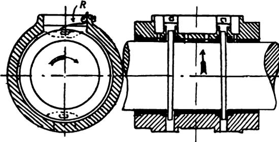
FIG. XII.—24. Bearing for Shaft with two fixed Oiling Rings.
