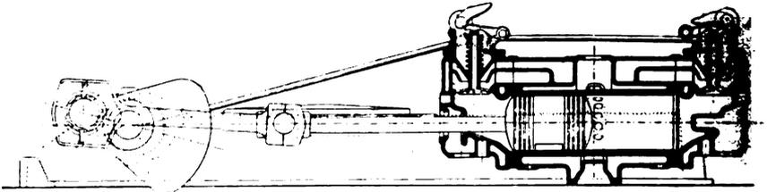
FIG. VIII.—8. Sectional elevation, Mather & Platt Engine (Koerting type).
