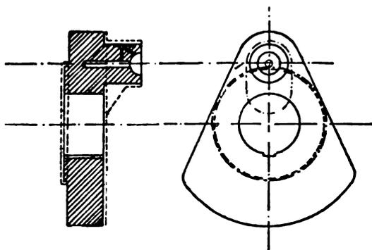
FIG. XIII.—20. Side Crank. Snow Steam Pump Works.
