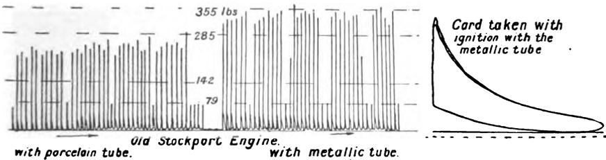
FIG. X.—5. Variation of explosion pressures with "tube" ignition.
