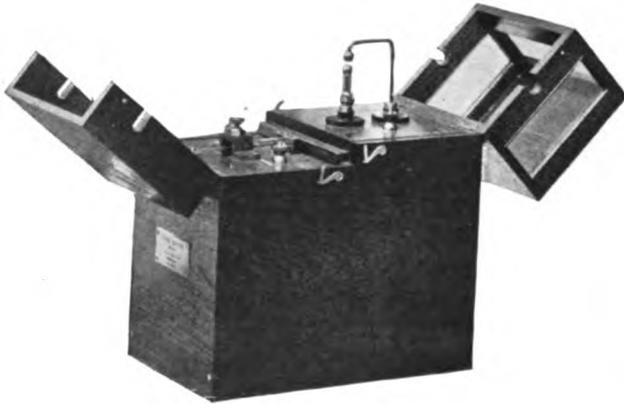
FIG. X.—26. Lodge high-tension ignition apparatus.
