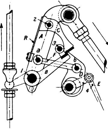
FIG. VIII.—12. Governor Trip Gear, Oechelhäuser Engine.
