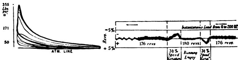
FIG. XV.—33. Diagrams and Tachograph from 200 H.P. double-acting Engine.
