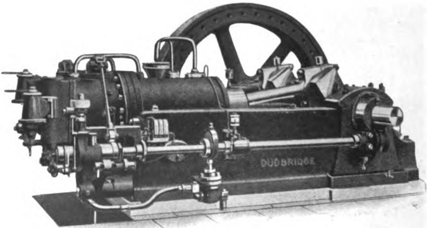
FIG. V.—8. Two-cylinder, twin, single-acting, four-cycle Dudbridge Engine.
