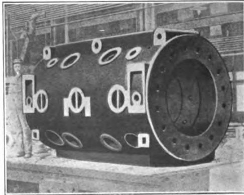
FIG. XII.—55. Cylinder Casting, Allis Chalmers Co.
