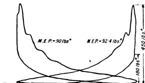
FIG. X.—50. Indicator diagram from double-acting Deutz Engine.
