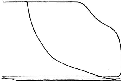
FIG. XIV.—19. Resistance Diagram from throttle-governed Engine, working load.
