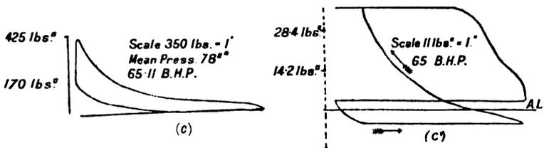
FIG. XV.—30. "Power" and "Resistance" Diagrams, full load.
