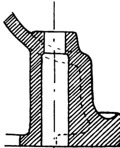
FIG. XII.—16. Boss for Foundation Bolt, with Solid Sheathing.
