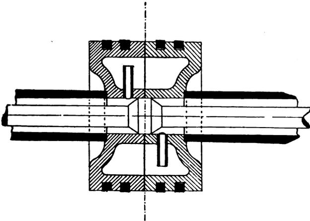
FIG. XIII.—57. Snow Steam Pump Works Piston and Rod.
