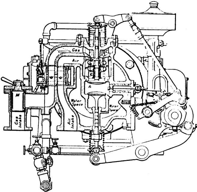
FIG. XIII.—75. Valve Gear of Olds Gas Power Co.'s Engine.
