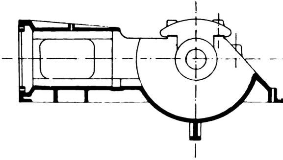
FIG. XII.—6. Frame suitable for various Cylinder Combinations (Reichenbach).
