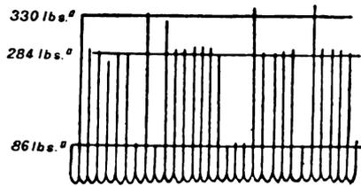
FIG. XV.—6. Explosion Record, rich mixture, after cut-out stroke.
