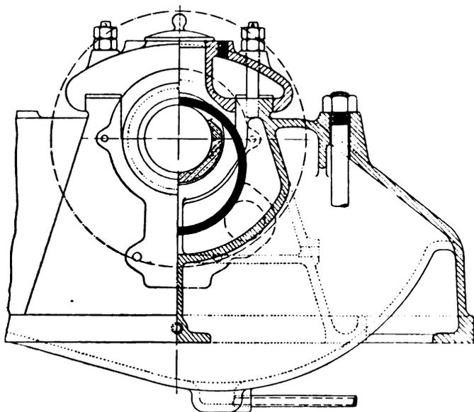
FIG. X.—42. Ring lubrication of main bearings.
