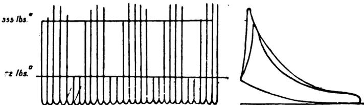
FIG. XV.—4. Explosion Record, weak mixture, after cut-out stroke.
