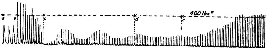
FIG. XV.—29. Explosion Record from throttle-governed Engine.
