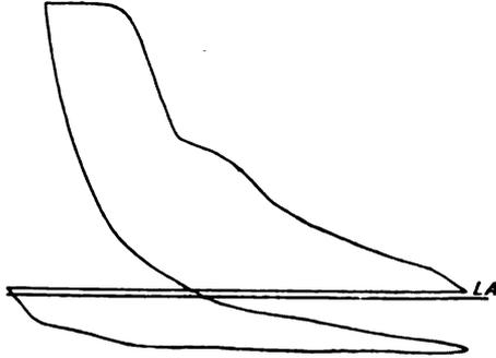
FIG. XIV.—18. Resistance Diagram from throttle-governed Engine, light load.
