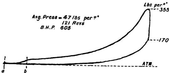
FIG. VIII.—11. Representative indicator diagram from Oechelhäuser Engine.
