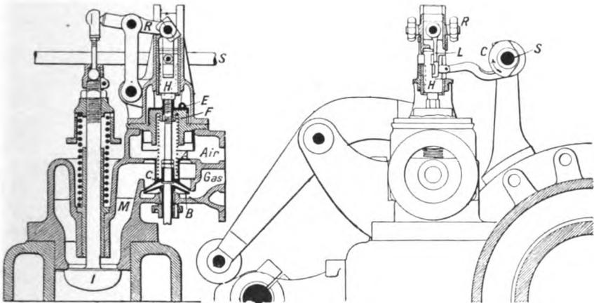
FIG. XI.—47. Snow Steam Pump Co.'s Governing Device.
