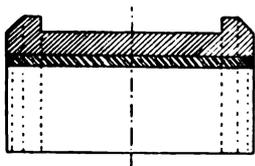
FIG. XII.—19. White-metal lined Bearing after cooling.
