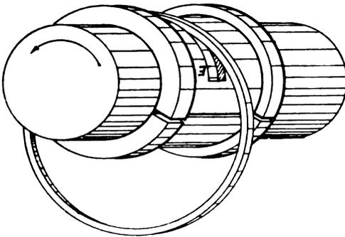
FIG. XII.—22. Shaft in Bearing, with Oiling Ring.
