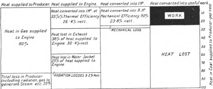
FIG. VII.—1. Thermal Balance-sheet of Marine Gas Engine.
