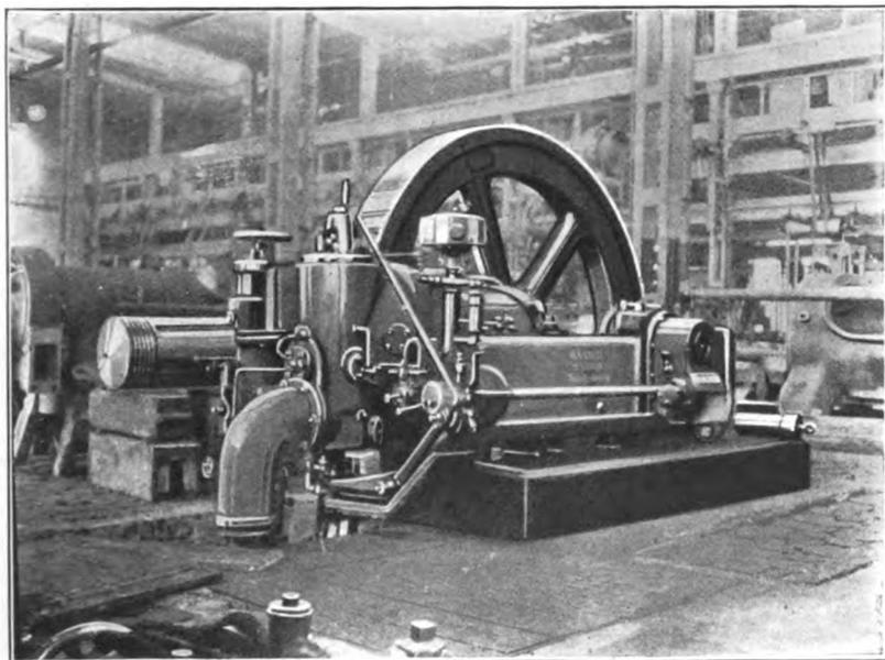
FIG. IV.—29. Nürnberg 60 H.P. single-acting, four-cycle Engine.
