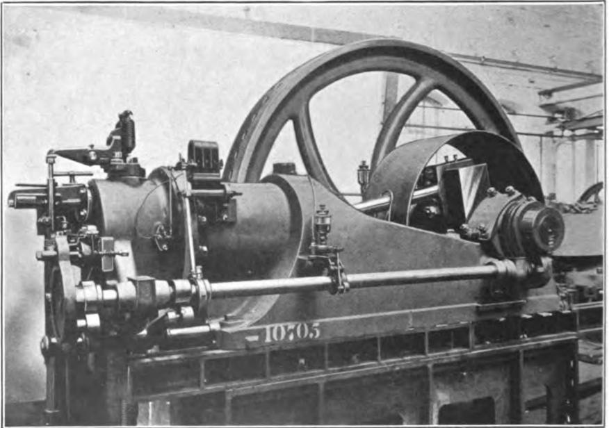
FIG. XIII.—73. Valve Gear of medium power Hornsby-Stockport Engines.
