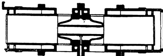
FIG. XII.—41. Section of Cylinders, Dingler.
