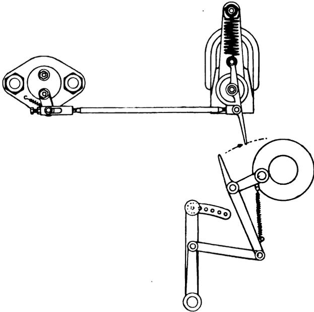
FIG. X.—17. Magneto mechanism, D. Stewart & Co.
