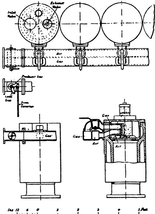
FIG. VI.—17. Mixture Regulation Device, Crossley vertical Engine.
