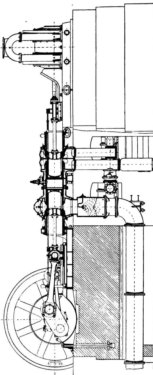
FIG. VIII.—15. Longitudinal section, Oechelhäuser Engine, with Blowing Cylinder.
