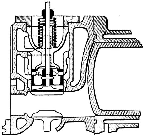
FIG. XII.—76. Combustion Chamber of Nürnberg Engine.
