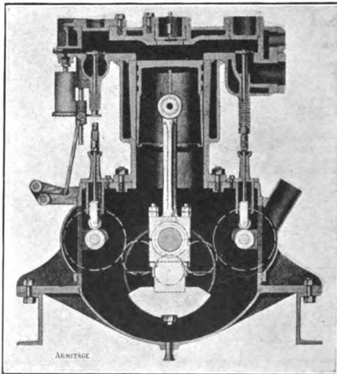
FIG. VI.—11. Transverse section, Gardner (enclosed) vertical Engine.
