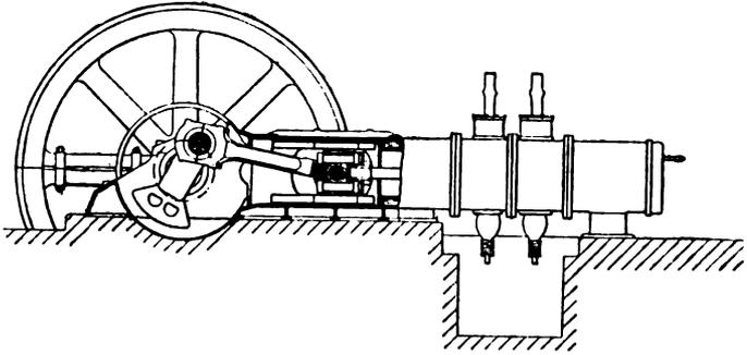
FIG. IV.—15. Dingler Gas Engine, part sectional elevation.
