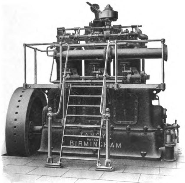
FIG. VI.—18. Three-cylinder, Tangye vertical Engine.
