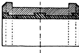
FIG. XII.—20. White-metal lined Bearing, with Dovetailed Grooves.
