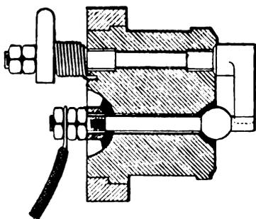
FIG. X.—9. Section through Sparking Plug (Winterthur).
