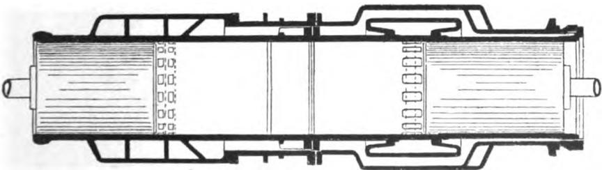
FIG. XII.—37. Section of Cylinder, Oechelhäuser Engine.
