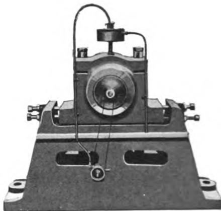
FIG. XII.—30. Hornsby Outer Bearing and special Oiling Device.
