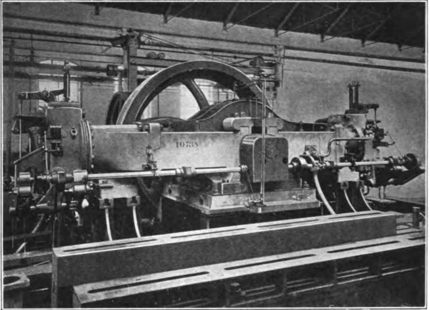
FIG. V.—7. Two-cylinder, *cis-d-cis*, single-acting, four-cycle Hornsby-Stockport Engine.
