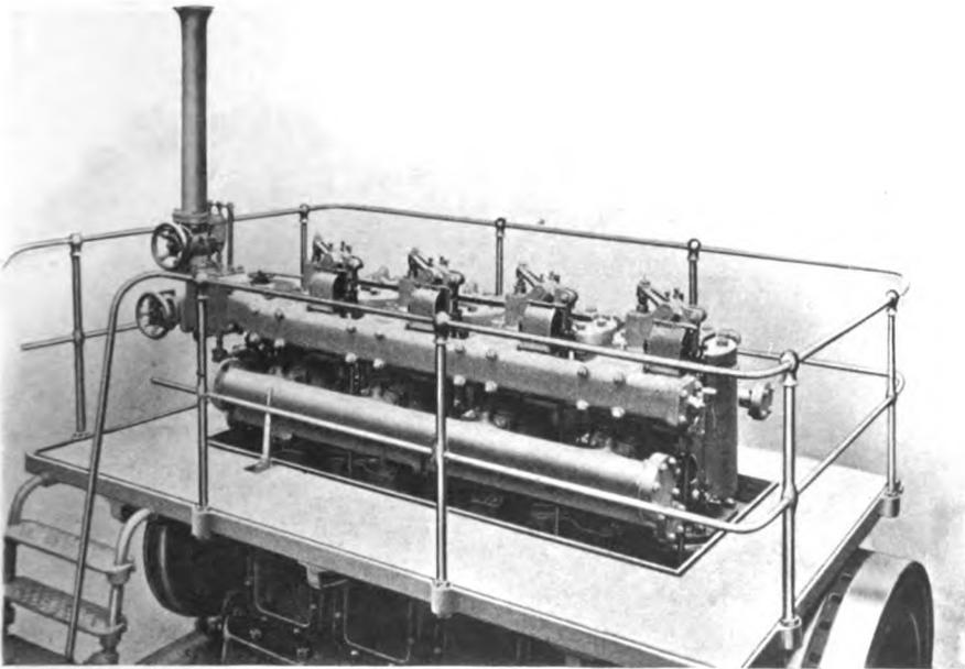
FIG. VI.—14. Cylinder-heads and valve gear, Campbell vertical Engine.
