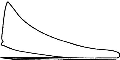
FIG. XIV.—10. Indicator Diagram showing faulty Cord Adjustment.
