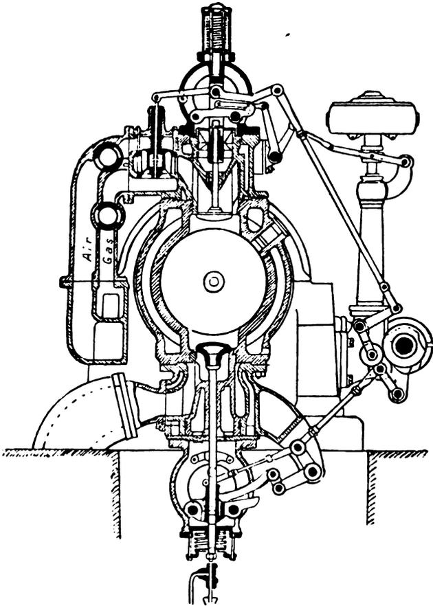
FIG. XI. 32. Governing Device, Otto-Deutz double-acting Engines.
