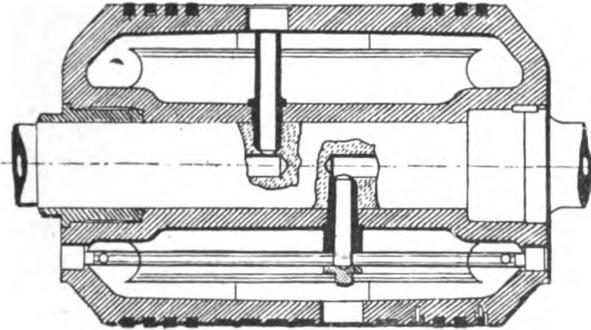
FIG. XIII.—50. Koerting water-cooled Piston.
