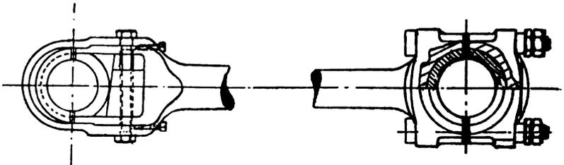
FIG. XIII.—27. Connecting Rod Ends.
