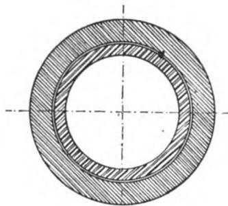
FIG. XII.—18. White-metal lined Bearing after cooling.
