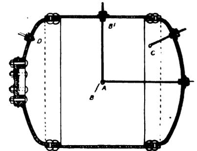
FIG. X.—2. Sectional drawing of Explosion Cylinder (Hopkinson's experiments).
