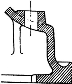
FIG. XII.—15. Boss for Foundation Bolt, with Stiffening Web.
