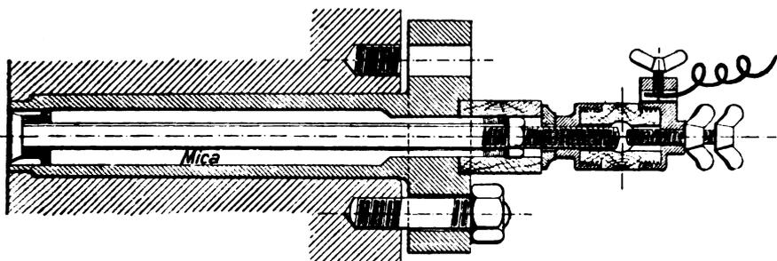
FIG. X.—25. High-tension Sparking Plug for Lodge ignition system.
