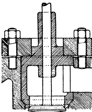
FIG. XII.—88. Removable Valve Seat with separate flange.
