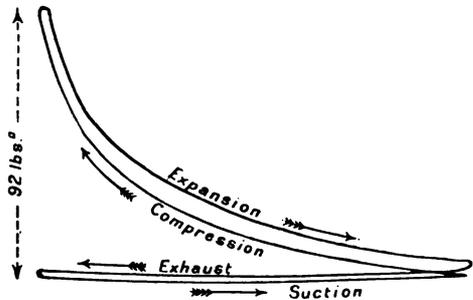
FIG. XIV.—17. Compression Diagram from Engine with hot walls.
