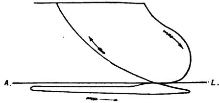
FIG. XV.—12. Resistance Diagram showing Scavenging by Fluid Inertia.
