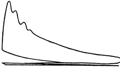
FIG. XIV.—13. Indicator Diagram taken with unsuitable Spring.
