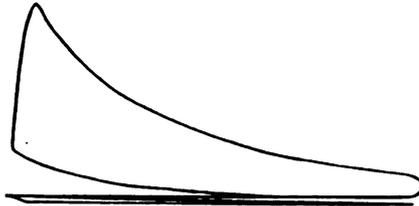
FIG. XIV.—12. Typical Indicator Diagram—Four-cycle Engine.
