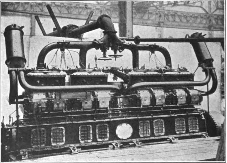
FIG. VII.—8. Koerting two-cycle, multi-cylinder Engine, for Submarine Vessels.
