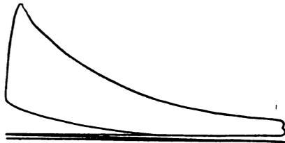
FIG. XIV.—11. Indicator Diagram showing faulty Cord Adjustment.
