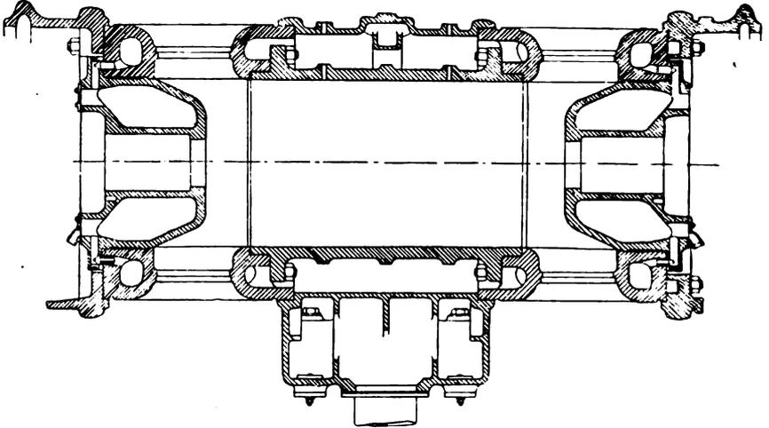
FIG. XII.—46. Section of Cylinder, Gasmotoren Fabrik Deutz.
