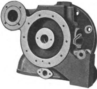
FIG. XII.—82. Breech end Casting of Schmitz Engine.
