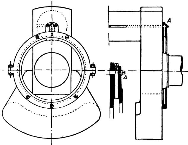
FIG. X.—39. Crank-pin Lubricator.
