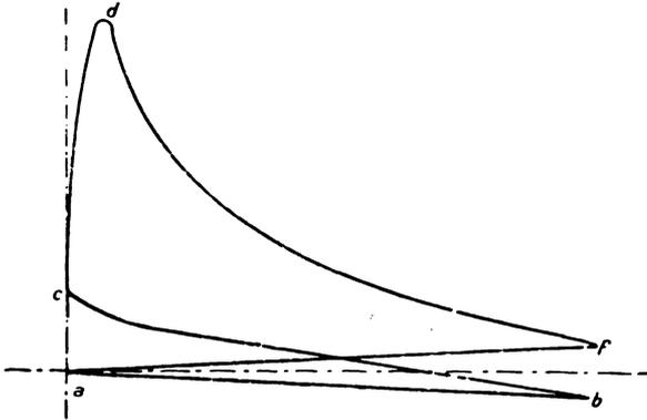
FIG. VIII.—1. Indicator diagram, illustrating four-stroke cycle.
