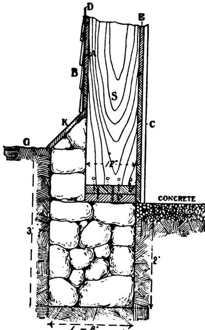
Fig. 167. Foundation of silo. Bottom of silo one foot below ground. (Cook.)
