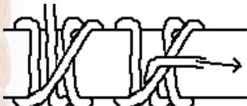
The best simple hitch for lengthwise pull. It needs to be laid very carefully and pulled firmly before loading. Never use it for right angle pull, for it will spill.
