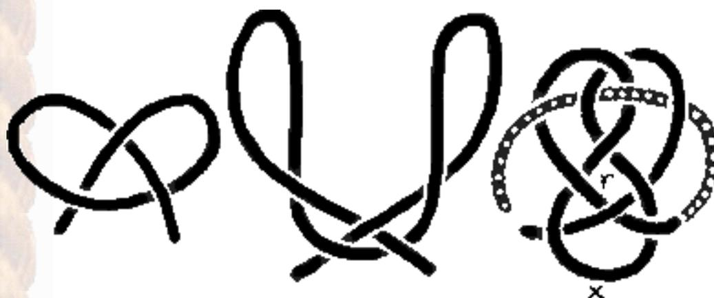
Start with a half knot and lengthen the two bights. Twist the bights to lock them (this will produce a regular over and under weave). Lay one bight over the other (check that the sequence is correct by examining the rectangle r) Take one end and lock the bights as shown.
