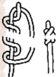
If you make more than two turns in the overhand knot it will be fatter. (But hardly stronger.) In twined rope it is important to work up the knot very carefully. (It will not only look neater, it wil prevent 'kinking' which will weaken the rope even more!)
