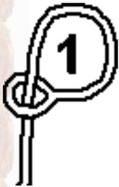
There are three basic ways to make a noose. The first way is running the 'tail' of rope through a fixed loop on the end of that same rope. This may be a spliced-loop or a knotted-loop like the bowline. (In fact the [bowline](#) is used very often as the running loop by sailors.) The simple noose itself is used as a running knot for swift running loops.
