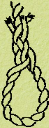
A method of putting a permanent eye in the end of a rope. The strands are unbraided, a loop of suitable size formed and the three strands are spliced or worked in and out of the rope, usually under and over. Three "tucks" are normally taken.
