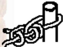
This is a remarkably useful knot. It is adjustable AND trustworthy. Each sailor should know how to tie this knot in any circumstance. Especially to tie himself to a rescue rope thrown to him in the water. On the lifeline he has to hold the loose end securely to the standing part. This gives a good grip and a useful goal in this critical situation (HOLD!)
