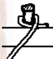
Although this is probably the simplest knot of all, you have to be a skilled knot-tyer to know how to tie and use it in a safe way. The loose end of the rope is nipped against the object and the standing part. The best nip is obtained against an edge or shoulder. If the load is released and the standing part shaken, the hitch is spilled instantly.
