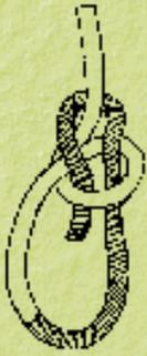
The most useful and one of the simplest ways of putting a fixed loop in the end of a rope. It is easy to tie and untie, it never slips nor jams and has a high breaking strength.
