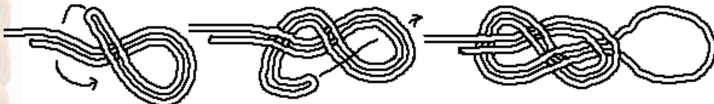
The double eight is a knot used by climbers. It is easy to tie and safer as the bowline. There is a discussion whether there should be a stopper at the end of the loose end or not. Speed of (un)tying is a safety factor itself.
