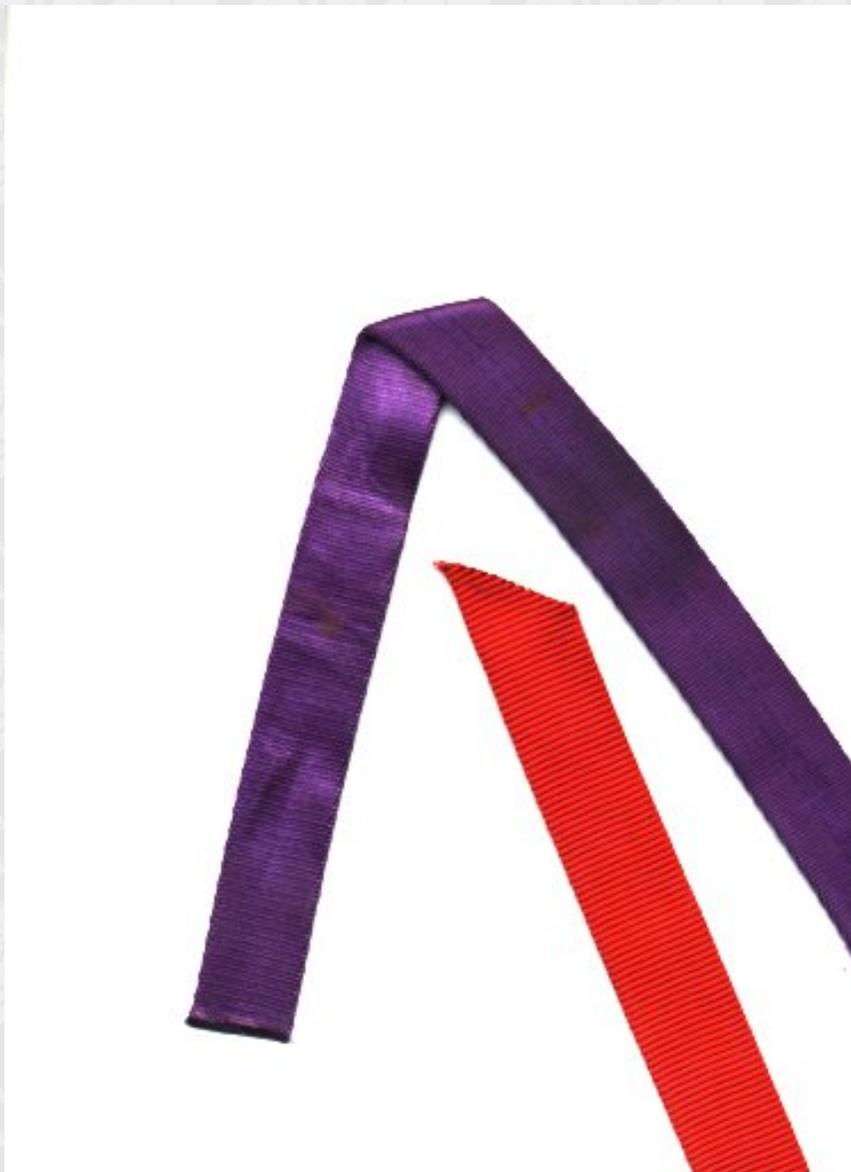
First place one end of webbing within a bend in the other end. NB: the different colors here are to illustrate technique, this knot is most often tied with one length of webbing.
