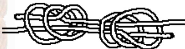
This is the double-stopper knot with the [Double Overhandknot](#) as a base. In fact you tie two [strangle knots](#) round the standing parts of both ropes. It is best to tie two counter-image strangle knots. With equal knots
