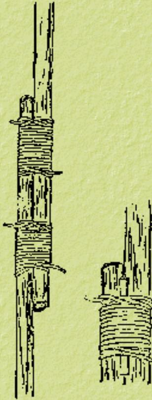
Used to lash two poles together (constructing a flagpole)
