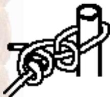
This brother of the midshipmans Hitch is just a bit less important. This is because it tends to jam. When jamming is desirable, this knot is o.k., as when work will be left unattended. Ashley states it was used by cotton brokers in New Bedford to tie their cotton samples they took from mill to mill. The packages could be opened and closed at will, and still be secure when left alone at travel.
