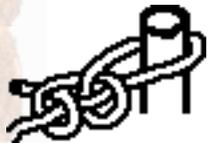
The two half hitches is used for tying a rope with a right-angle pull to a pole or ring. It should be constant under load. (Not under constant load). It does not jam. If the object you tie it on has a small diameter it is better to use the "Round Turn with Two Half Hitches". This is the same knot but with an extra turn round the
