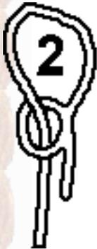
The second way to make a noose is to tie a running knot (a simple knot or hitch) round the standing part of the rope in a way that pulling on the knot-side closes the loop. This is the most common way for making nooses. It makes the loop to close almost as easy as a noose using a fixed loop as a running knot.
