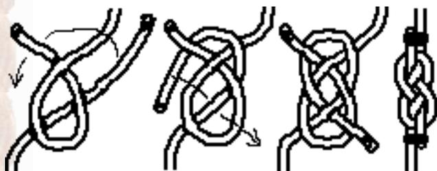
Also known as Full carrick Bend, Sailor's Knot and Anchor Bend. Beware! There are not many knots with so much wrong drawings as this bend. The ends have to be on opposite sites and the crossings always are alternating up/down/up/down... The Carrick Bend is one of the best knots. Ashley states it is possible the nearest thing we have to a perfect bend.
