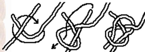
If you want to tie two thin yarns to each other you use a wever-knot. The one shown here is the same as the Sheet Bend. If the yarn is slippery use an [Overhandknot](#) on the ends before tying this knot. If this ends up into a too bulky knot you need another wever\_knot.
