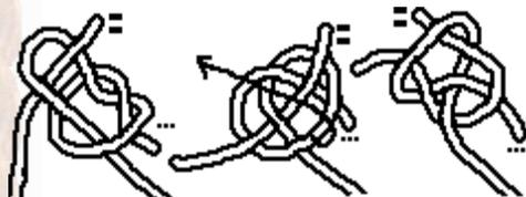
With the simplest noose you can catch an end and capsize the knot to a sheet bend. Be careful. without practicing you have a 50% change of catching it wrong. Also, (as always) working up the knot properly is important.
