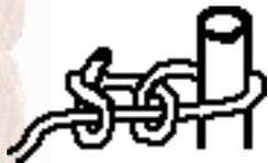
This knot is used to tie guy-ropes to tent-poles. But it is inferior to the [Tautline Hitch](#). The only reason I have included it in the elementary hitches is because its topology places it there. I see no use for it. (Please let me know if you know an application where this knot is the best knot to use.) A keen eye will recognize a capsized Reefknot in it.
