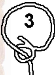
The third way is to tie a running knot in a way that pulling the knot is opening the loop. I only know one practical application for this way of tying this noose: for tying the rope to a yo yo, with the eight as running knot. But in packing bags and loads you will find it sometimes as an intermediate loop. It is also often the result of tying the running knot the wrong way.
