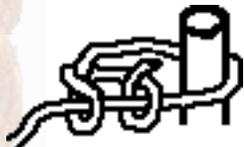
The Lobster Buoy Hitch is almost as secure as the Buntline Hitch, but more easy to untie. It is used to tie timber.
