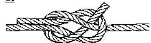
left-hand rope. (2) Reeve the running part of the right-hand rope through the eye of the bight in the left-hand rope. (3) With the right-hand running part take a bight around the running part and the standing part of the left-hand rope. (4) Pass the right-hand running part over the left-hand standing part, (5) under the right-hand rope, and (6) over the standing part of the left-hand rope. (7) Pull tight.
