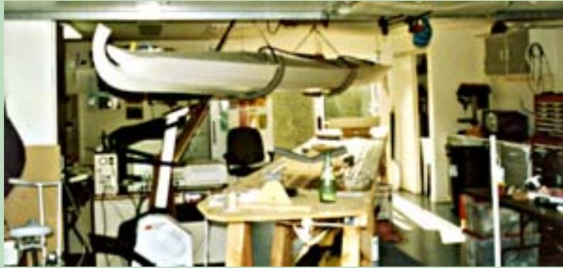
The most critical part of this operation is to have the frame supports cut out and precisely placed on the strong-back (work bench)
