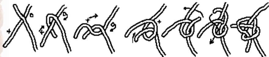
This way of tying is for connecting equally sized ropes to each other. When the ends are connected you have the [Bowline Knot](#). You have to try to take the first 'steps' as one simple clockwise turn of your wrist. So practice...
