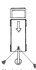
Erecting the poles using a truck. With the tip of the pole resting on the tailgate, the truck slowly backs up, angling the pole upward. Use skids to prevent damage to the edge of the hole, and guide ropes to control the pole as it goes up.
