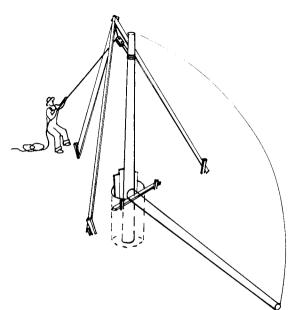
Erecting the poles using a block and tackle. The pulley may be attached to an overhanging tree, if convenient. For maximum embedment strength, use wooden skids as shown to prevent damage to the walls of the hole.
