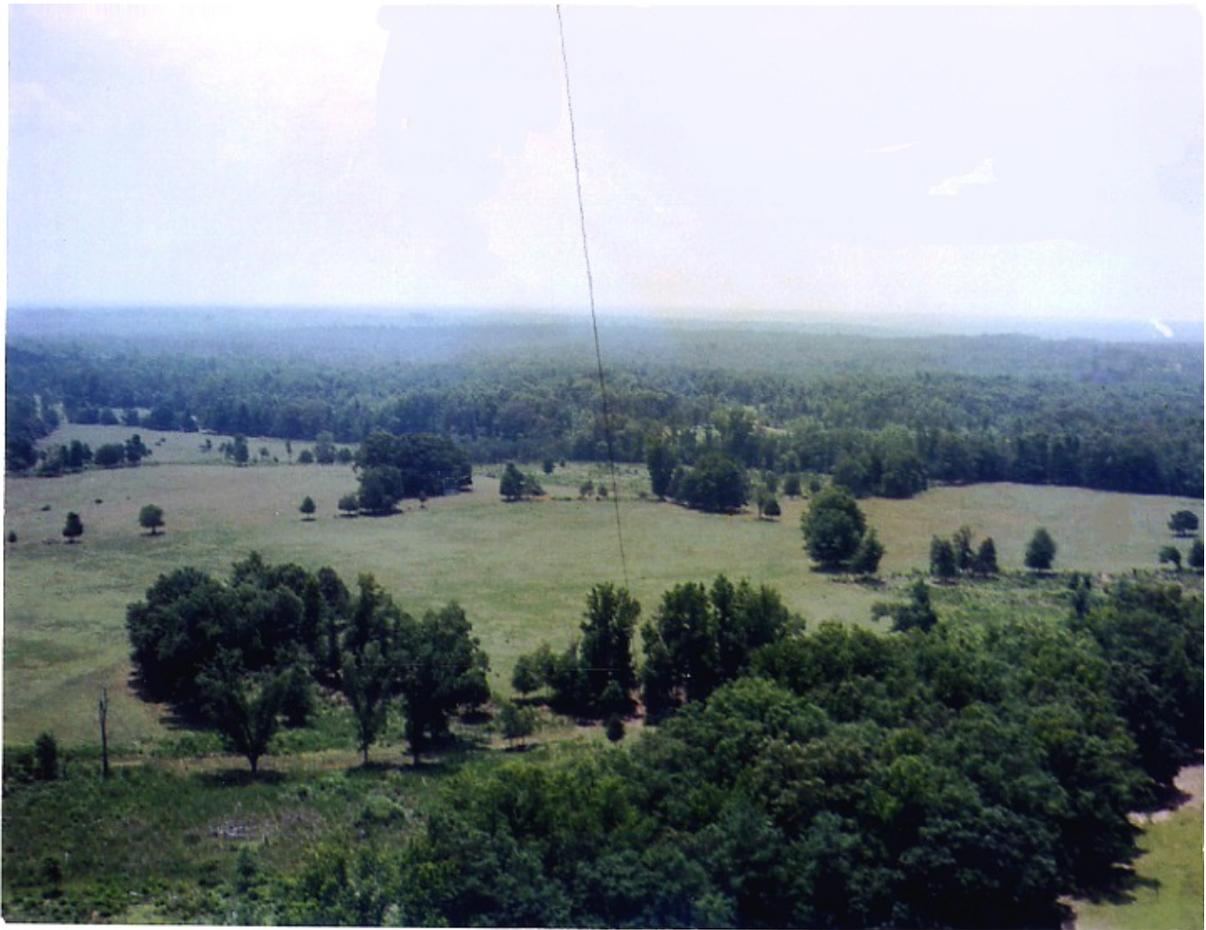
Ground height is about 800 feet above sea level, but the important thing for VHF and UHF is the ground slowly rolls away in three directions. The effective height above average terrain for your view for the next 20 miles is around 300-feet, even though you are only 250ft above ground.
