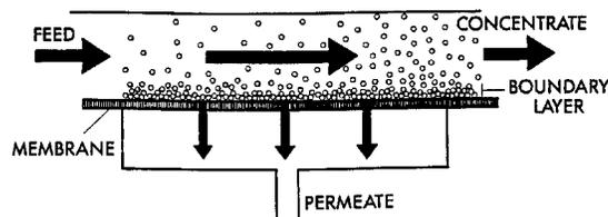
There are four general categories of crossflow membrane filtration: microfiltration, ultrafiltration, nanofiltration, and reverse osmosis.
